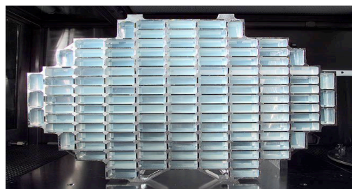
Figure 4. Stardust aerogel collector (NASA/JPL).
